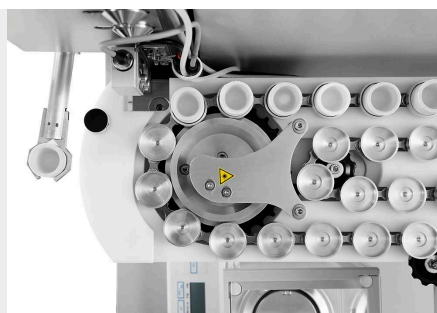
Placing sample in autoloader and analysis
