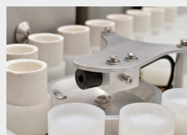
Autoloader with acid-resistant plastic crucible holders
