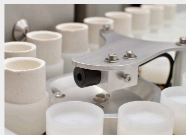
Autoloader with acid-resistant plastic crucible holders
