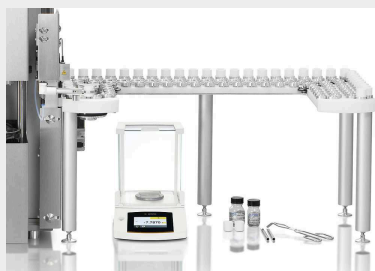
Autoloader with 130 crucible positions
