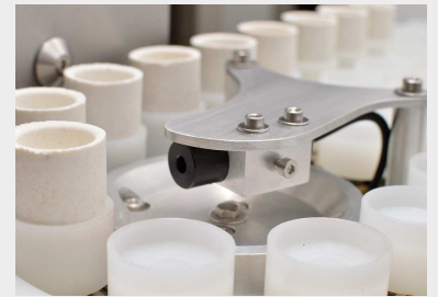
Autoloader with acid-resistant plastic crucible holders
