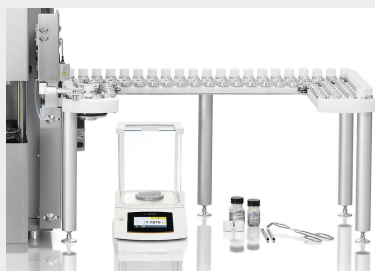
Autoloader with 130 crucible positions
