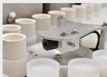
Autoloader with acid-resistant plastic crucible holders
