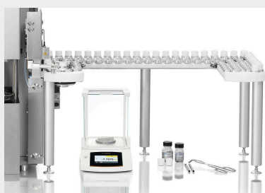
Autoloader with 130 crucible positions
