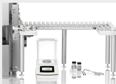
Autoloader with 130 crucible positions
