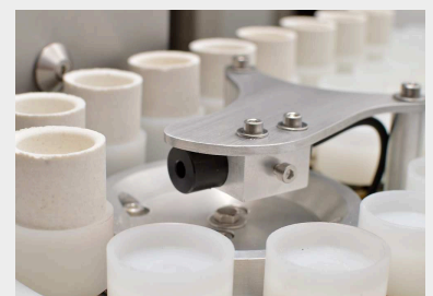
Autoloader with acid-resistant plastic crucible holders
